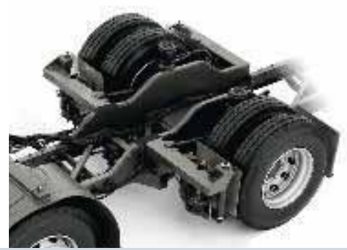
The driven axle is a drop-centre axle available with a wide selection of ratios.
