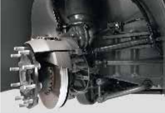
The front axle is of the drop-centre type, offering no less than 54 degrees of turning angle.
