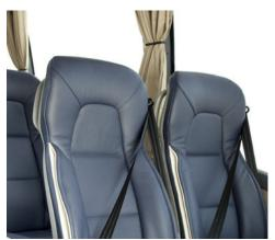
A safe journey. The Volvo 9900 is designed to provide a safe journey for everyone. The seats feature deformation zones and can be equipped with three-point seat belts, booster cushions and integrated rear-facing child seats.
