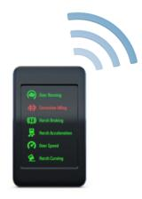
**I-Coaching assists the driver** to drive more safely, fuel efficiently and comfortably. It gives instant feedback on parameters such as over-revving, excessive idling, over-speed and harsh curving, helping the driver improve performance.
