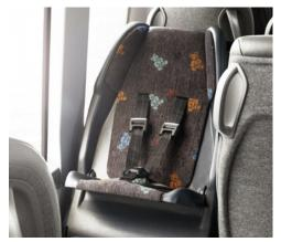
**A safe journey.** The Volvo 9700 is designed to provide a safe journey for everyone. The seats feature deformation zones and can be equipped with three-point seat belts, booster cushions and even integrated rear-facing child seats.
