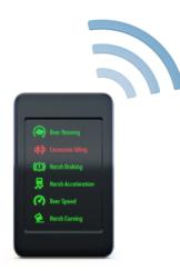
I-Coaching assists the driver to drive more safely, fuel efficiently and comfortably. It gives instant feedback on parameters such as over-revving, excessive idling, over-speed and harsh curving, helping the driver improve performance.
