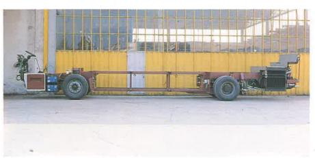
The classic chassis can take different engines; independent front wheel suspension, disc brakes and triangular frame rear suspension.
