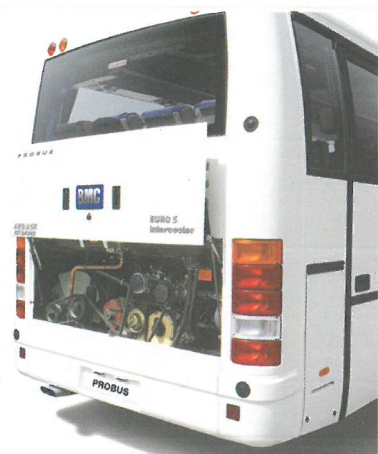
285 PS Euro 5/EEV Cummins rear fitted engine and manual/automatic gearbox options for increased ride comfort
