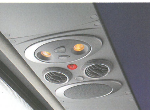
Personal comfort controls: individual reading lights and air flows
